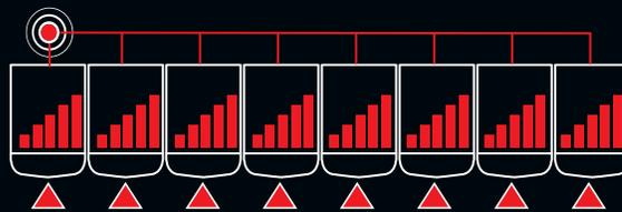
This feature optimizes the modulation capabilities of the Boiler Plant while evenly distributing run time across all cascaded boilers. Every 24 hours the SMART SYSTEM automatically shifts the 1st boiler on role to the next in the sequence, distributing run time equally.
