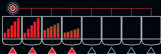
The "lead" boiler modulates with demand to capacity. As demand increases, additional boilers fire and modulate to capacity. This continues, with additional boilers firing and modulating to capacity until all units are operating. Every 24 hours, the SMART SYSTEM automatically shifts the lead boiler role to the next in the sequence, distributing lead-lag runtimes equally.
